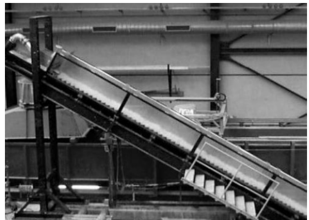
Figure 2 : LCH stepped spillway channel (André 2004)
