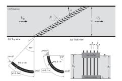
Fig. 2: Geometric and hydraulic rack parameters of modified curvedbar racks (a) rack top view, (b) bar shape top view, (c) side view
