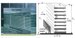
Fig. 2: (a) Laboratory experiment on a HBR with bottom and top overlays (b) Definition sketch for governing HBR parameters
