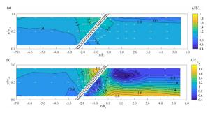
**Fig. 4**: Measured flow field of  $U/U_o$  at MCR configuration  $\alpha = 30^\circ$ , s = 50 mm (a)  $\beta = 45^\circ$  and (b)  $\beta = 90^\circ$ .
