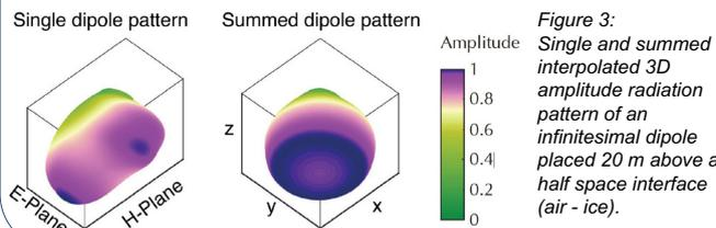
Figure 3: Single and summed interpolated 3D amplitude radiation pattern of an infinitesimal dipole placed 20 m above a half space interface (air - ice).
