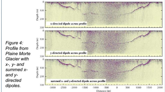
Figure 4: Profile from Plaine Morte Glacier with x-, y- and summed x- and y-directed dipoles.
