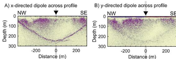
Figure 2: Comparison of ground-based pulseEKKO PRO 25-MHz Profiles
