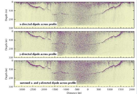
Figure 4: Profile from Plaine Morte Glacier with x-, y- and summed x- and y-directed dipoles.
