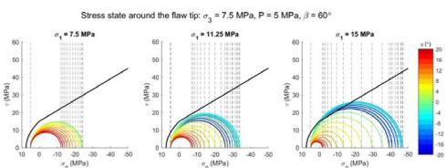
Fig. 4: Effect of an increase of vertical stress on the stress state around the tip of a pressurized flaw leading to shear failure.
