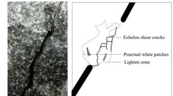
Fig. 6: Crack scenarios with crack types and coalescence categories observed in the uniaxial experiments. Biaxial experiments only show scenario 3.
