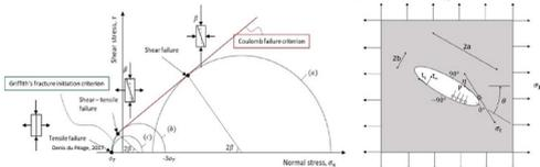
Fig. 3: Failure envelope and Mohr circles corresponding to tensile and shear failure (left). Elliptical flaw in an elastic plate with biaxial stress (right).
