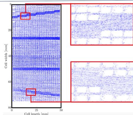
Velocity field of the full field of view, obtained by the temporo-ensemble method. Enlargement of velocity field in the dead-end fracture embedded in the low-permeability matrix (top-right) and the dead-end fracture embedded in the high-permeability matrix (bottom-right).
