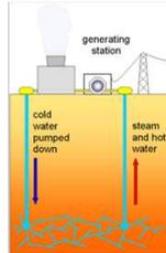
Fig. 1: Enhanced Geothermal System <http://climateresearch.blogs.pot.com/>.
