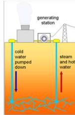
Fig. 1: Enhanced Geothermal System <http://climateresearch.blogs.pot.com/>.
