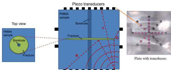
Schematic of the transducer layout and different arrival modes.
