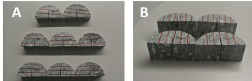
Figure 1: A) and B) presents the two endmembers with the foliation aligned ( $\varphi=90^\circ$ ) and normal ( $\varphi=0^\circ$ ) to the artificial notch.
