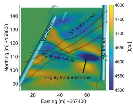
Fig. 4: Seismic tomography with interpolated shear zones.
