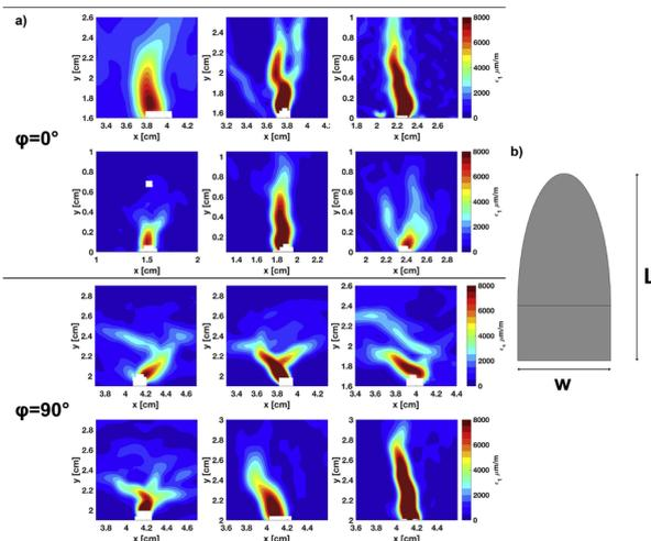
Figure 3: (a) The contours of maximum principal strain showing the FPZ shape at peak load for the configurations  $\varphi = 0^\circ, 90^\circ$ . (b) The FPZ at the peak load is idealized schematically as a semi-elliptical region with the width of  $W$  and the length of  $L$  (Dutler et al., 2018).
