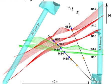
Figure 1: Experimental volume at GTS (top view): Injection boreholes (black lines), HF injection intervals (orange cylinders), HS injection intervals (blue cylinders), the shear zones along with the far field stress state ( $\sigma_1 \sim 13.8$  MPa, plunging to the East with  $30-40^\circ$ ,  $\sigma_3 \sim 8$  MPa, sub-horizontal North-South,  $\sigma_2 \sim 8.5$  MPa, Krietsch et al., 2018)
