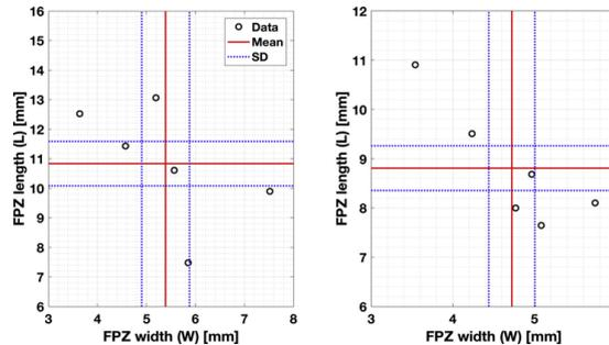
Figure 5: The measured values for the FPZ width ( $W$ ) and length ( $L$ ) for two cases of  $\varphi = 0^\circ$  and  $\varphi = 90^\circ$ . The mean values of the six tests are shown by red line, while the blue pointed line show the standard deviation. The results are taken from the fully formed FPZ, i.e. at 70% of pre-peak load for  $\varphi = 0^\circ$  and 90% of pre-peak load for  $\varphi = 90^\circ$  (Dutler et al., 2018).
