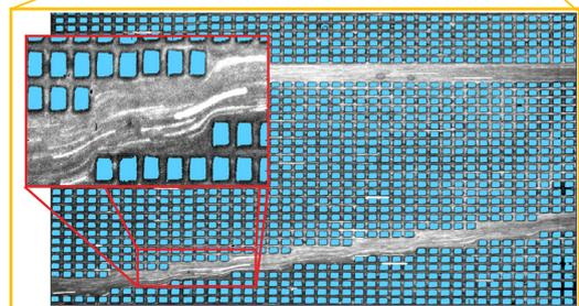
A time-lapse image of particle trajectories, captured during a time interval of 25 sec. The whiteness quantifies the particle density. Blue patches indicate the masks which are applied to exclude regions of impermeable pillars during the PIV calculations.
