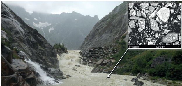
Fig. 1: Mountain stream transporting sediment (Wysswasser downstream of the Fieschergletscher, Valais; picture: VAW 2013) with microscope image of suspended sediment particles (IGT, ETH Zürich; Felix 2017).
