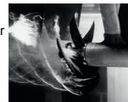
Fig. 6: Cavitating propeller model in a water tunnel experiment.
