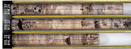
Fig. 2: Drill-core section of the Trigonodus Dolomit at the BEN borehole. The cm-dm scale cavities originate from the dissolution of eogenetic anhydrite nodules.
