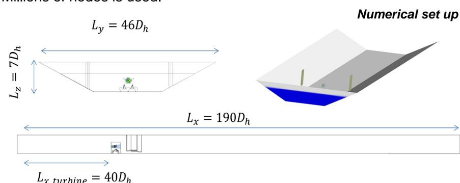
The numerical results have shown that the turbine has no impact on the available head of the Lavey powerplant. Moreover the Venturi effect of the duct and the specific design for the runner induce a strong acceleration of the flow inside the machine, as expected [1].
