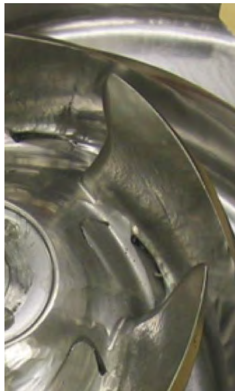
Fig. 1 – Depiction of an eroded open impeller (picture taken from [3])
