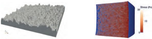
Fig. 2. Left: Generated rough surface. Right: stresses on the rough contact surface of a displaced cube. From [1].
