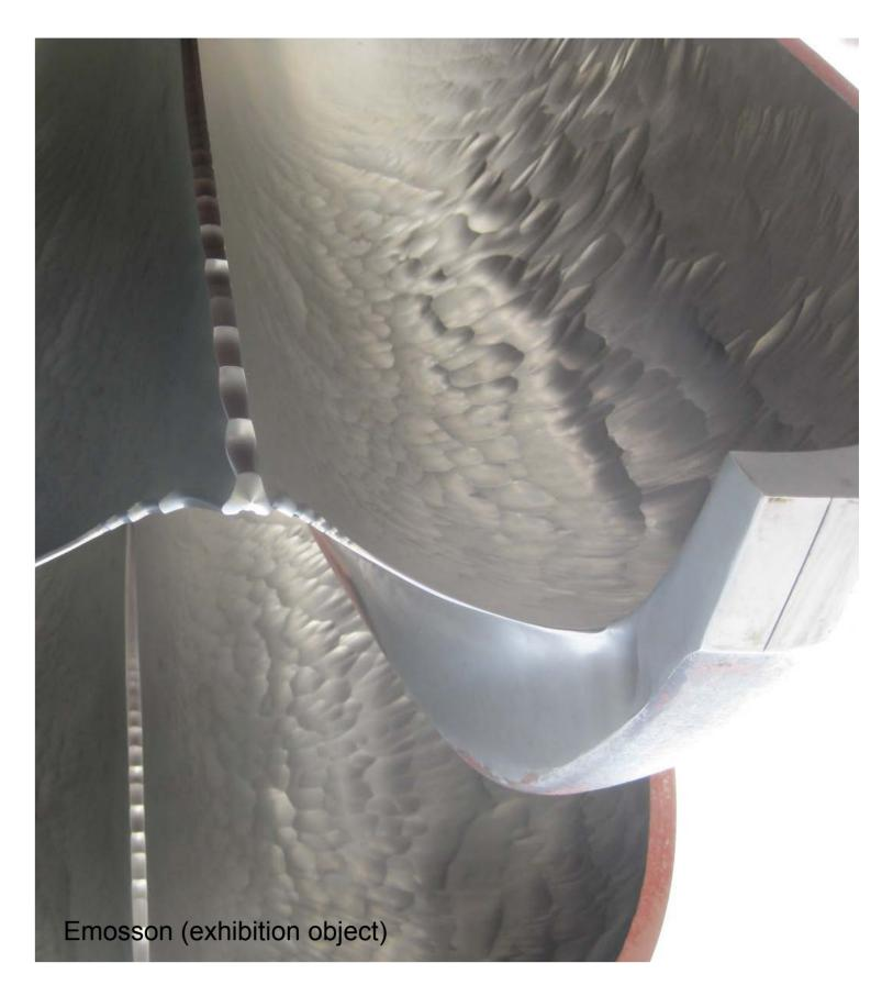
Fig. 2: Runner of Pelton turbine with abrasion damages
