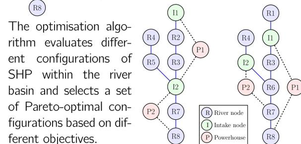
The optimisation algorithm evaluates different configurations of SHP within the river basin and selects a set of Pareto-optimal configurations based on different objectives.
