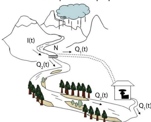
Schematics of SHPP; water is distributed at the node N following a given rule
