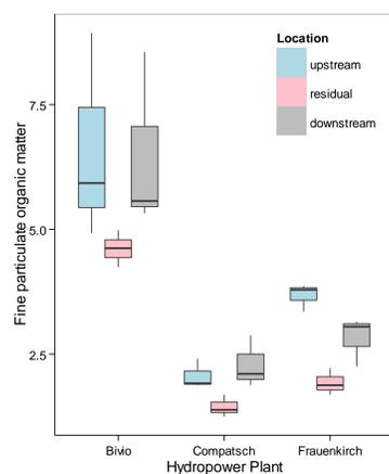
The sediment organic matter content was significantly lower in the residual flow reaches ( $p < 0.05$ ).
