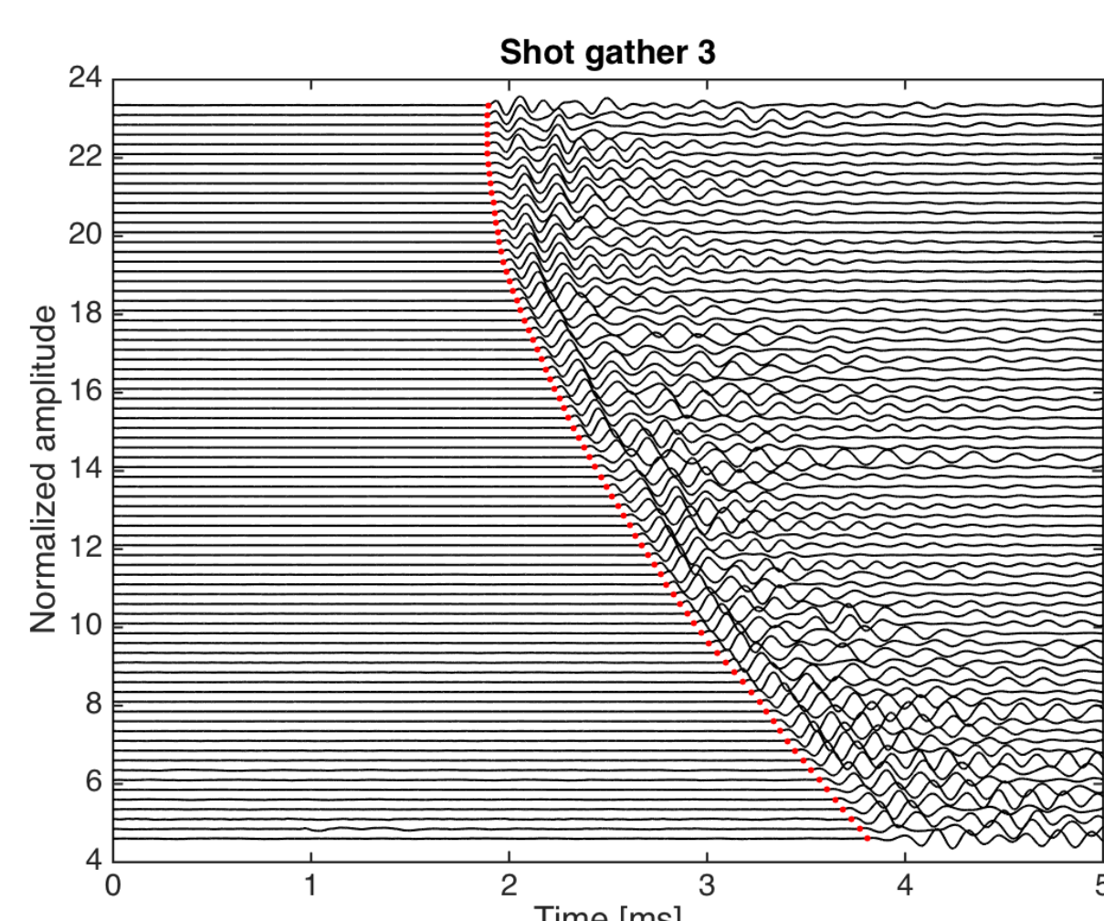
Tomography between FRI boreholes
