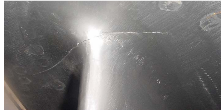
New Impeller Experienced Cracks at the Blade Roots due to Rotor-Stator Interactions in a 430 MW Modernized Pump-Turbine
