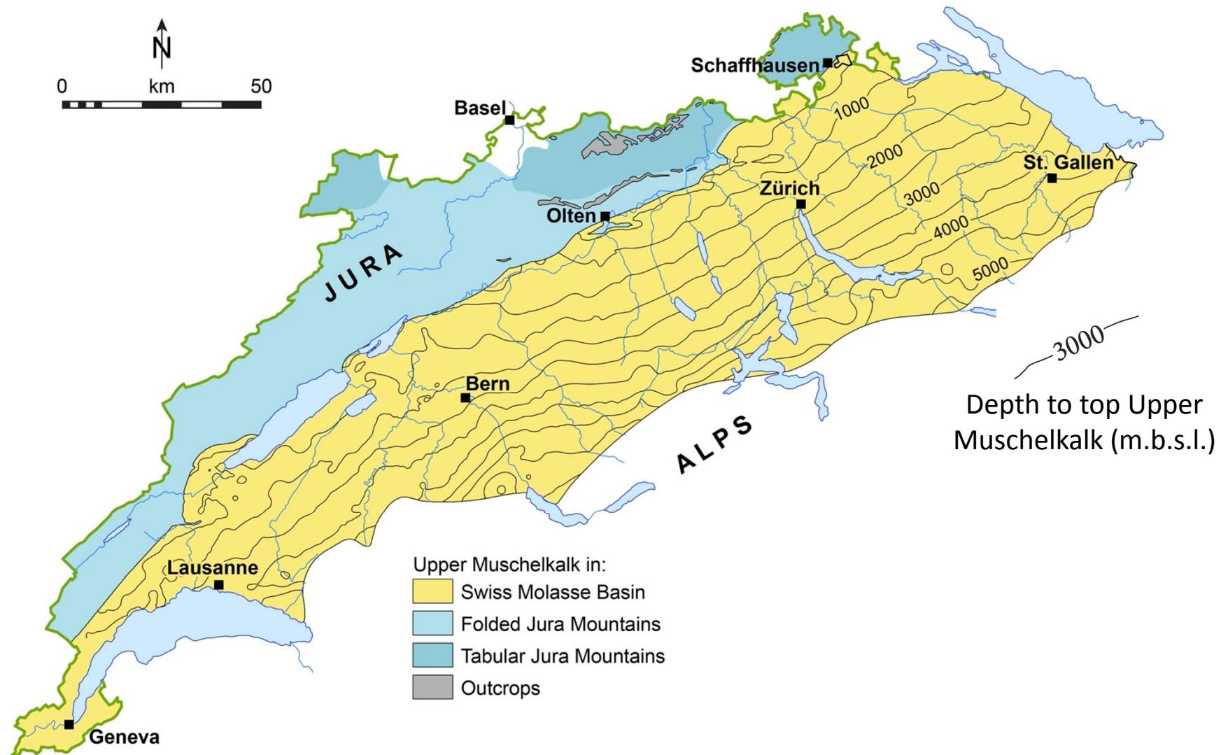
Upper Muschelkalk dolomite sealed by impermeable evaporite caprock
